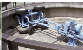
Driving tester (evaluates durability against being hit, assuming a 4-ton truck)
