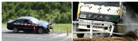
Performance verification using actual vehicle collision tests
